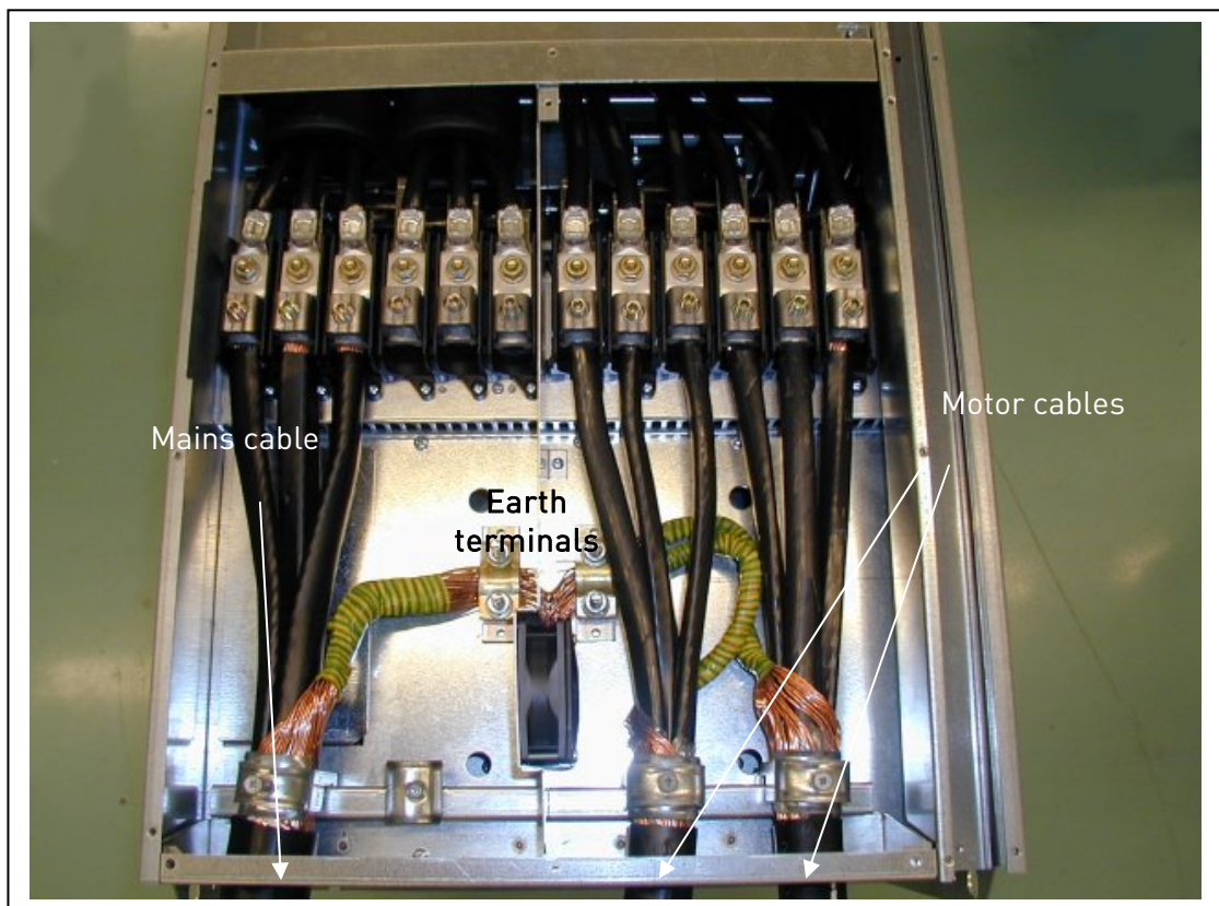
Figure 6-20. Cable installation in Vacon NXS/P, FR9
